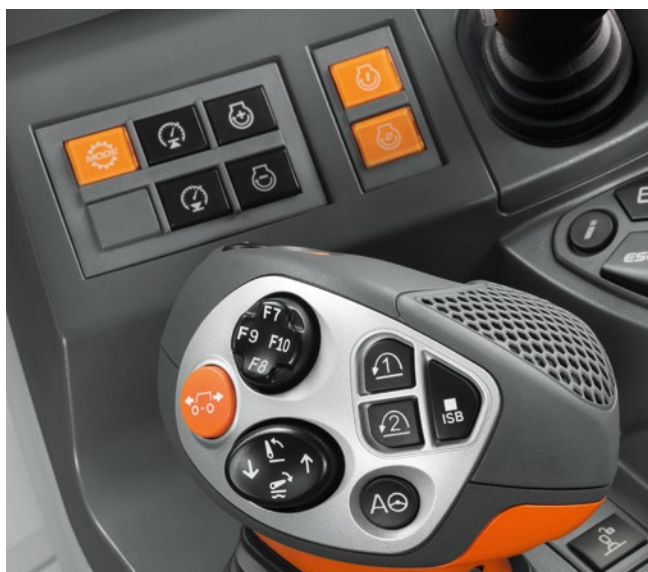
Engine droop setting for “Eco” and “Power”, and the engine speed memory.
