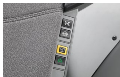
Switch to activate front axle suspension.
