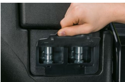
External battery terminals are within easy reach by the left-hand cab access ladder.
