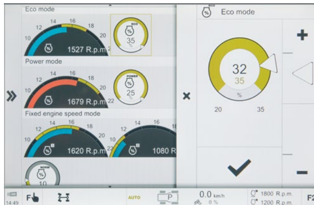
Engine droop setting for “Eco” and “Power”, and the engine speed memory.
